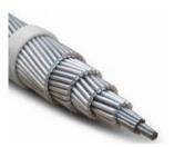
Designed to offer unique optimal strength for line design, these overhead transmission cables meet international standards including ASTM, BS, DIN, IEC, NFC etc. These are concentrically stranded conductor with one or more layers of hard drawn Aluminium wire on galvanized steel wire core which are coated with zinc with Class A Coating. The core can be single wire or stranded depending on the size of the conductors.
